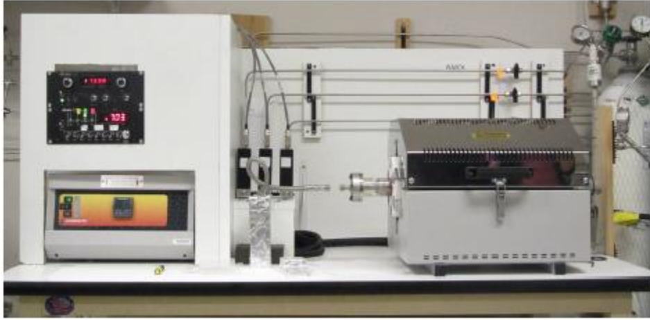
Figure 2.1 The home-built CVD graphene synthesis system
